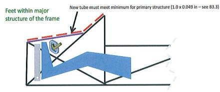
• T3.18.1 The driver's feet and legs must be completely contained within the Major Structure of the Frame. While the driver's feet are touching the pedals, in side and front views no part of the driver's feet or legs can extend above or outside of the Major Structure of the Frame.
